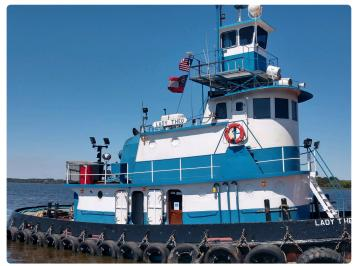
The Lady Theo is a versatile Model Bow Coastal Tug. It has an Upper House and a towing winch, which are both very helpful in tending dredges and mobilization of equipment on the ICW.
